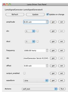
Cool, right? Using Python amazing introspection capabilities together with Feat annotations inside the driver, Lantz was able to build **on-the-fly** a Graphical User Interface for testing purposes.
